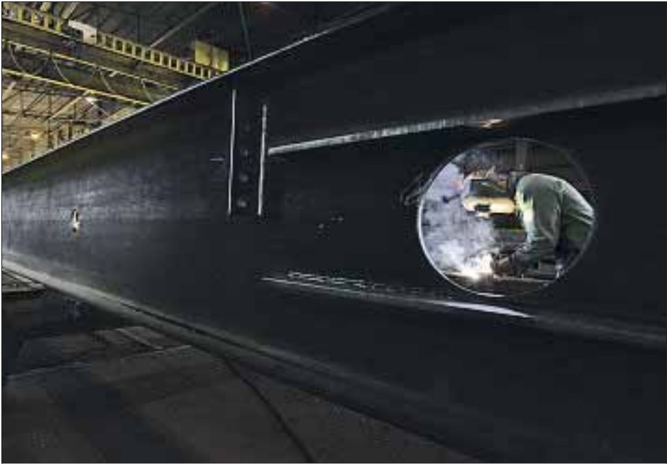
A WELDER attaches clips onto a steel column at Schuff Steel in Phoenix, where the Wilshire Grand project's steel was fabricated.
